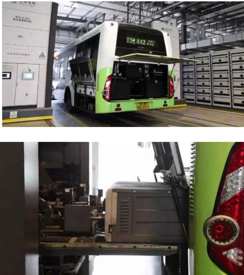
Figure 1: Swapping operations at the Xuejiadao Station in Qingdao
