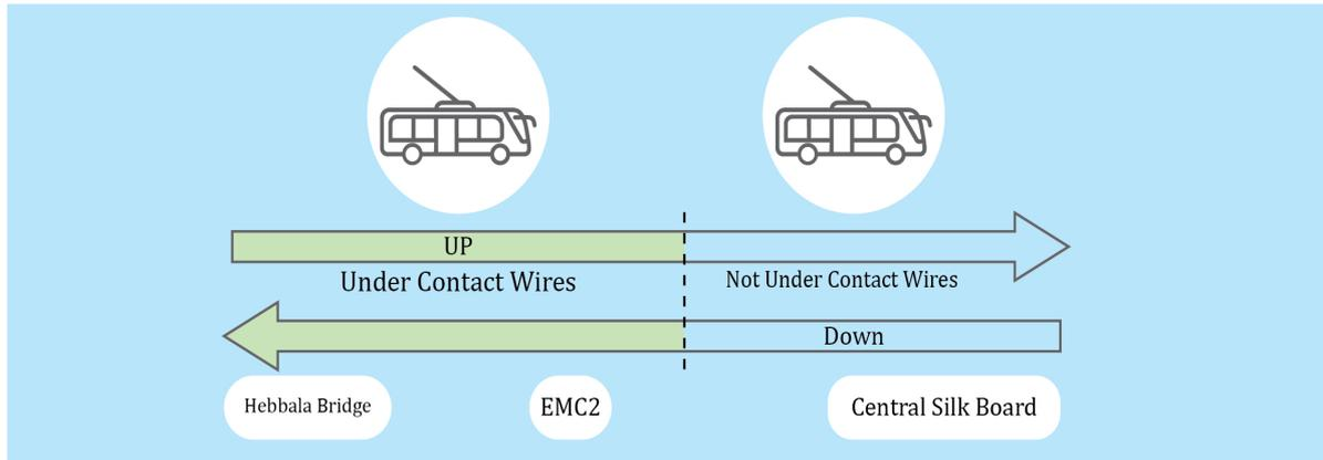
Figure 8: Overview of battery-assisted trolleybus operations on route V 500D
