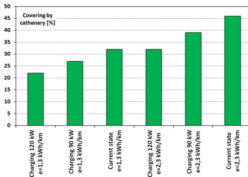
Figure 5: Minimum catenary coverage for various operating and charging conditions
