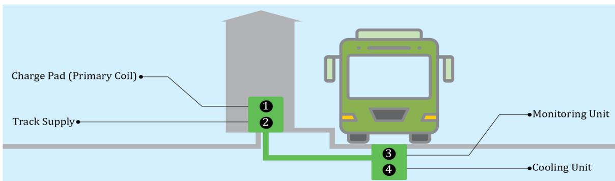
Figure 2: Schematic representation of induction charging
