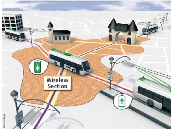
Figure 4: Schematic representation of in-motion charging systems
