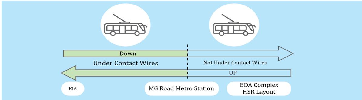
Figure 7: Overview of battery-assisted trolleybus operations on route KIAS 7A
